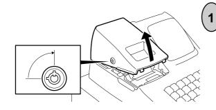
To remove the Printer Cover, insert the Printer Cover/Drawer key to the Printer Cover Lock, and then turn it 90° clockwise.
